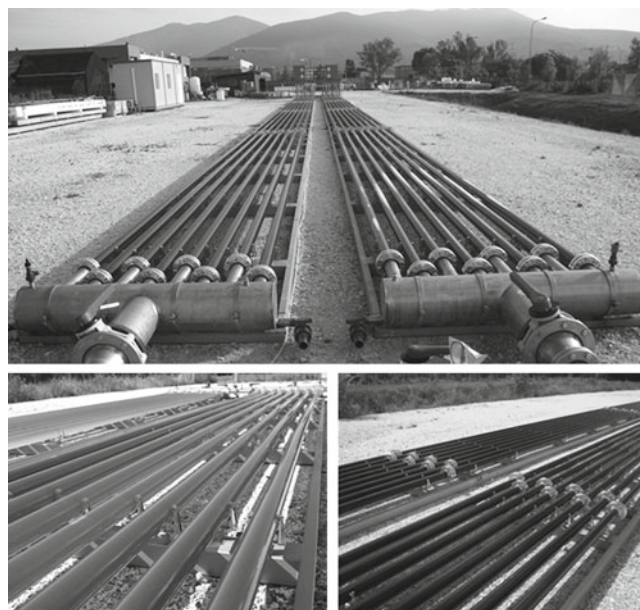
Fig. 7.8 Manifold tubular reactor developed by Sogepi S.r.l. (Milan, Italy) and F&M S.r.l. (Florence, Italy) (Photographs by the authors)
