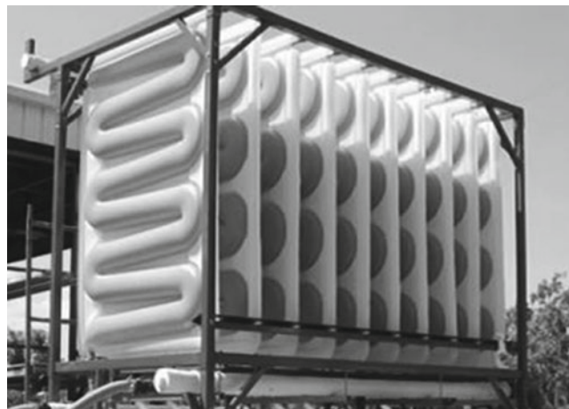
Fig. 7.6 Vertical plates developed by Renewed World Energies Corp. (USA) (Reproduced with permission from the company’s web site)
