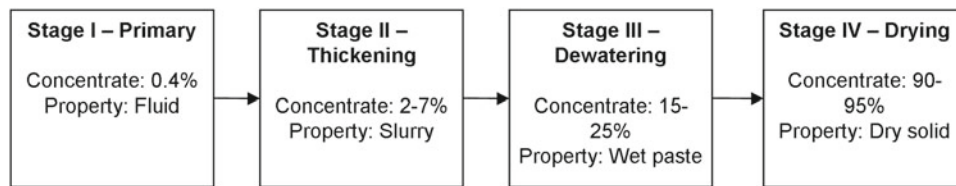
Fig. 10.2 Block flow diagram for the recovery of microalgae biomass, showing typical biomass concentration achieved and the physical state of the output stream
