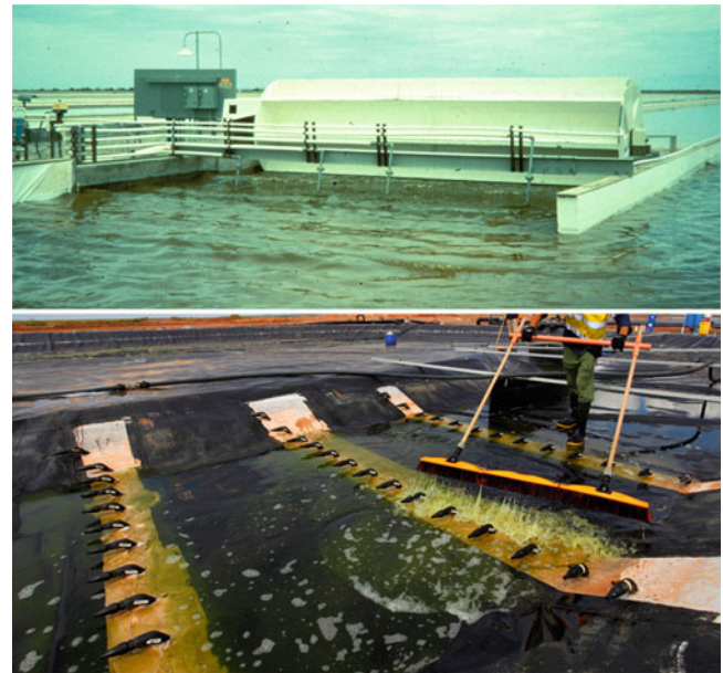
Fig. 8.2 Two types of circulation system for open ponds. Top : Paddle wheel; Bottom : Empty pond with jets at base of pond (Courtesy of Matt Caspari, Aurora Algae)
