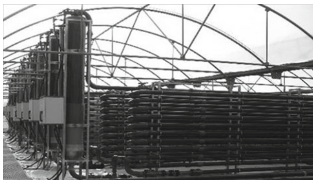
Fig. 7.7 Vertical tubular serpentine PBR developed by the Department of Chemical Engineering of the University of Almeria (Spain) (Courtesy of Prof. E Molina Grima)
