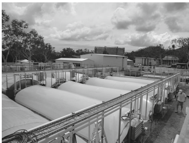
Fig. 7.9 Biological Algae Growth Systems (BAGS) developed by MBD Energy Ltd (Australia) (Courtesy of MBD Energy Ltd)
