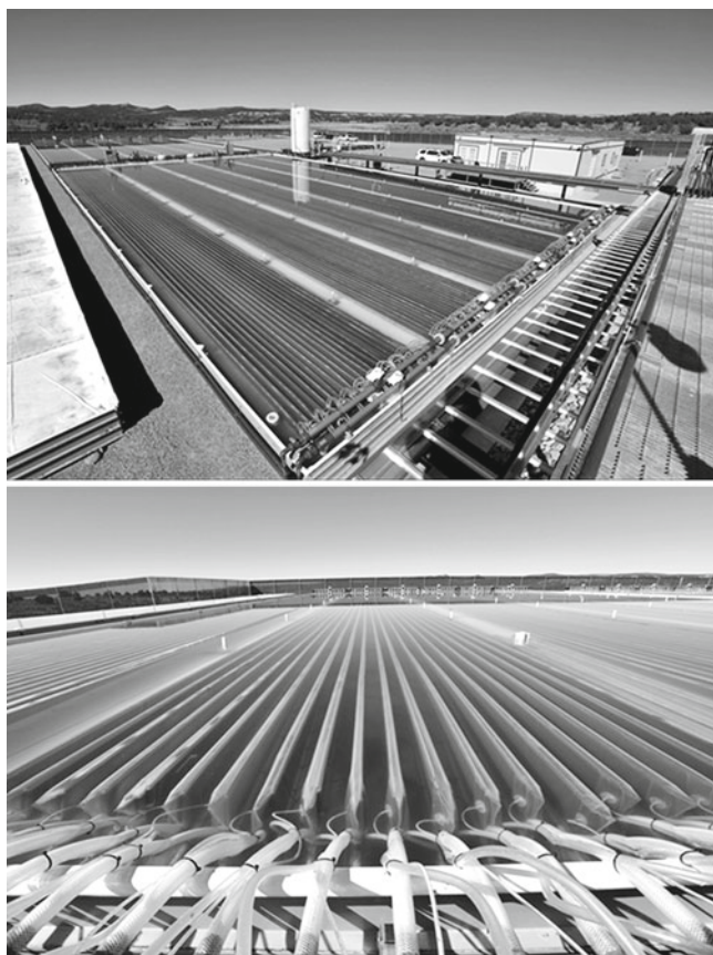
Fig. 7.3 Solix Biofuels® photobioreactor at the Coyote Gulch demonstration facility in Southern Colorado (USA) (Courtesy of Solix Biofuels®)
