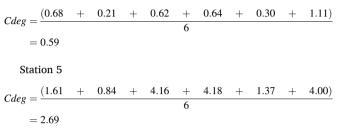
Station 4 showed a  $mC_{deg}$  value of 0.59, which also evidences a condition of very low contamination for this sampling point. Despite this, the  $mC_{deg}$  value for the Station 5 was 2.69 denoting moderate contamination in this region.
