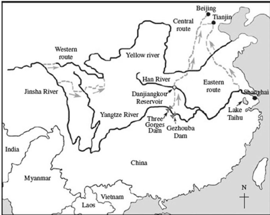
Fig. 2.4 The eastern, western, and central routes intended to transfer water from the Yangtze River to the north of China (Cite from Dudgeon 2011)
